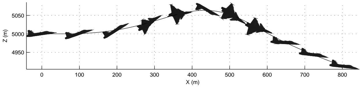
Figure 2. Simulated high angle of attack, high roll rate maneuver.
