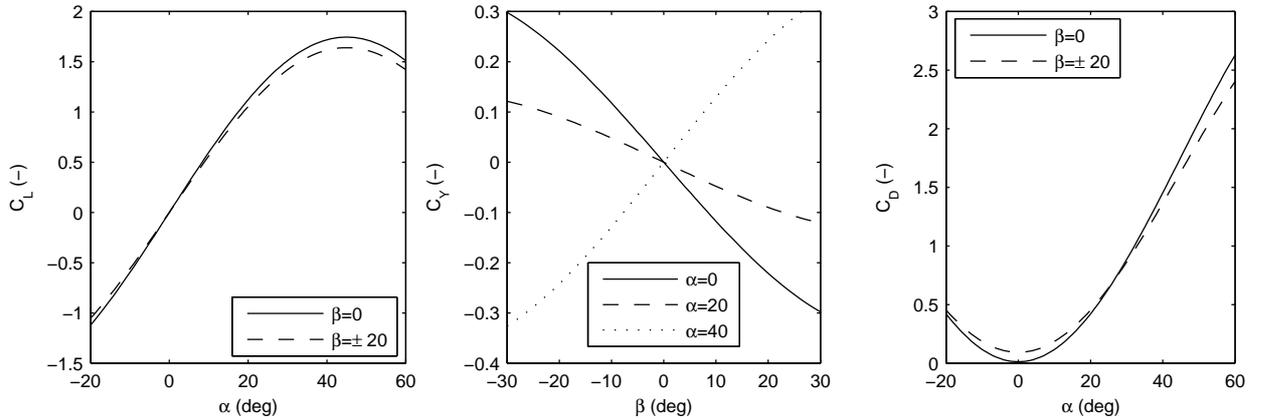
Figure 1. Aerodynamic coefficients for the lift force, side force, and drag force.
