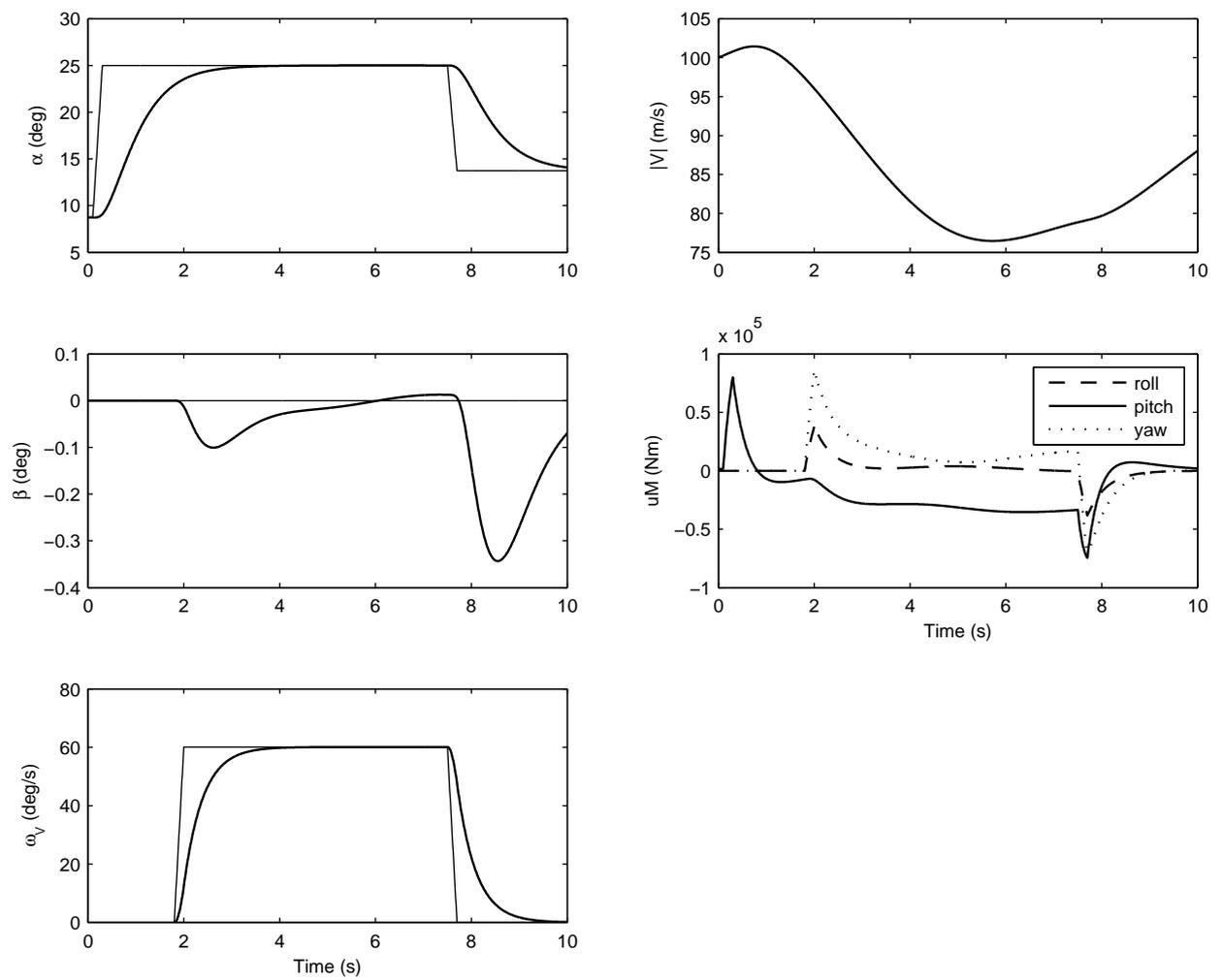
Figure 3. Aircraft variables (angle of attack  $\alpha$ , sideslip angle  $\beta$ , velocity vector roll rate  $\omega_V$ , total velocity  $|V|$ ) and controls (torque vector  $u_M$ ).
